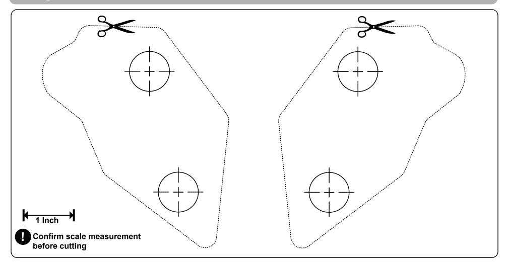
**Step Three:** Remove the top cover lids from the center top plastic. Cut out the drilling templates along the dotted line. Use tape to adhere the templates to the top cover lids. Using a center punch, mark the hole centers onto each top cover lid, then drill each hole using a 7/8" hole saw. Once drilled reinstall the top cover lids to the center top plastic. (Do not scale when printing, check scale with ruler before cutting)
