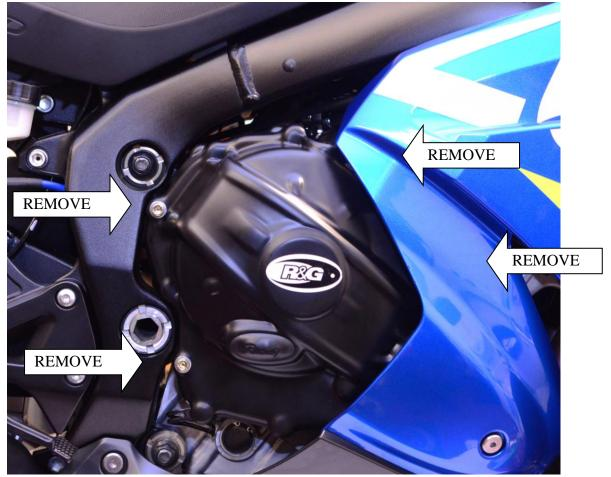
In this kit there should be: 1x Engine Case Cover (ECC0231R) 4x M6 x 40mm Long Cap Head Bolts 1x Racing Puck (SK0001SK (already fitted)). 2x PAL Nuts (already fitted).
