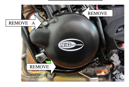
In this kit there should be: 1 x Engine Case Cover (ECC0139) 2 x M6x40mm CAP HEAD BOLTS 1 x M6x85mm CAP HEAD BOLTS
