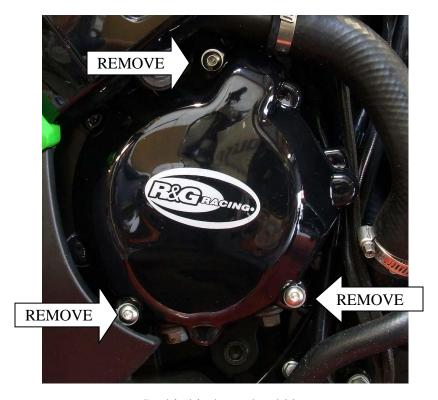
In this kit there should be 1 x Engine Case Cover (ECC0038) 3 x M6x45mm CAP HEAD BOLTS
