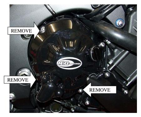
In this kit there should be 1 x Engine Case Cover (ECC0027) 3 x M6x50mm CAP HEAD BOLTS
