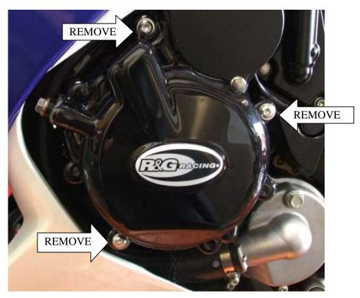
In this kit there should be: 1 x Engine Case Cover (ECC00001) 3 x M6x60mm long button head bolts
