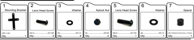
**Step One:** Remove the rectifier/regulator and horn/reflector assembly from their original locations. Use the M6 Bolts (#2), Washers (#3) and Nuts (#4) to mount the rectifier/regulator to the Mounting Bracket (#1). Next re-use the OEM hardware from the horn to bolt it to the Mounting Bracket (#1)
