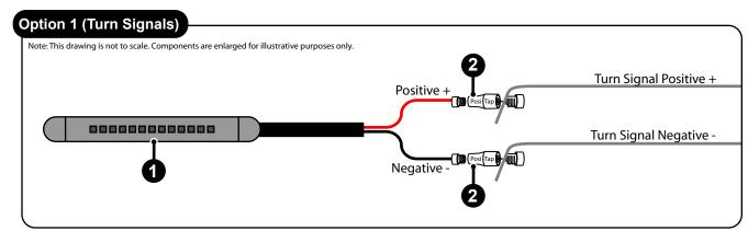
**Option One:** Locate the negative and positive leads for your right hand turn signal and use a Posi-tap to connect the leads from the LED strip. Repeat these steps with the left hand turn signal.
