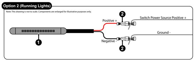
**Option Two:** Locate a switched power source and a ground, then use a Posi-tap to connect the leads from the LED strips.
